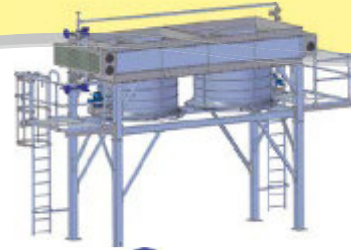
Air-cooled heat exchanger (Fin Fan)
